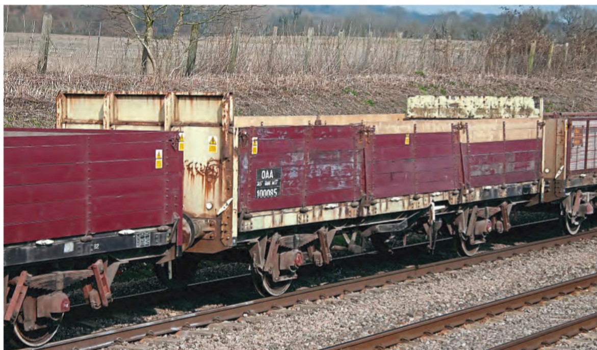
Another modification which could be included in a future run of the OAA model is the extended end modification as applied to No. 100085 which was recorded on March 1, 2004, painted in EWS maroon.
