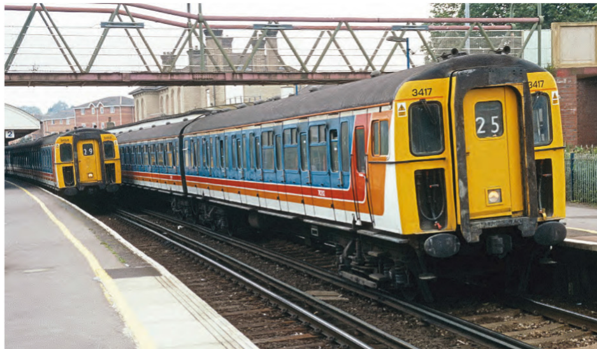
Services between Alton and Aldershot to Waterloo and Ascot were once dominated by 4-VEPs. No. 3417 and No. 3459 were noted on October 11, 2002. They are 'face-lifted' units with rebuilt MBSOs where the guard's van was reduced in size for a new passenger saloon which provided 18 additional seats.
