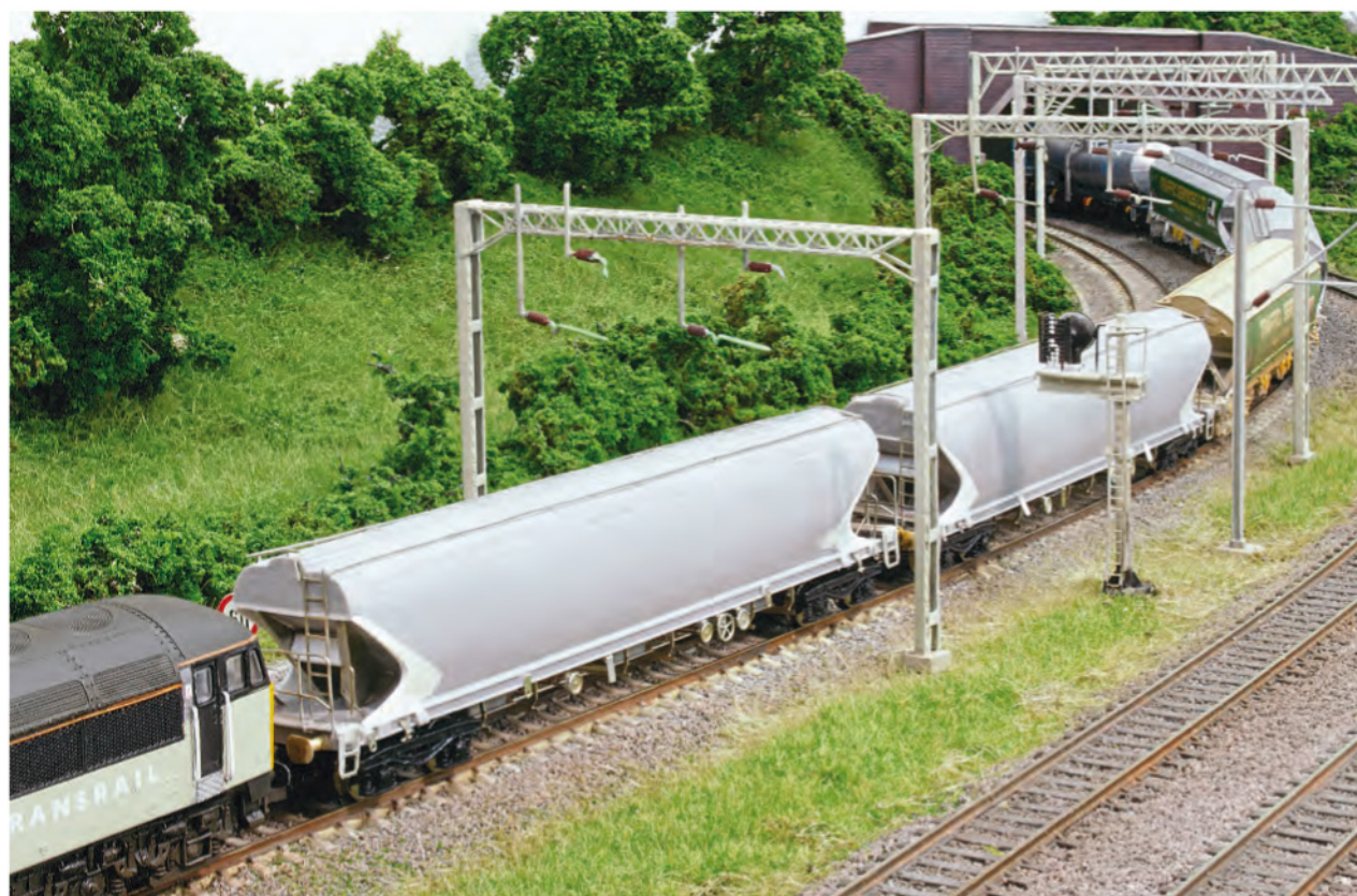
Test running of the SMD JIAs built from the N Gauge Society's kit. This test revealed that one ferry hook was interfering with a wagon bogie, tilting the wagon to one side. An important point to look for during tests which is simple to correct.
