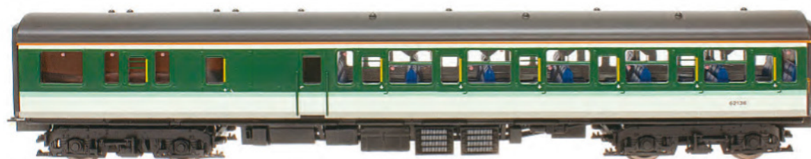
MBSO No. 62136 of Southern No. 3514. The motor block and drive bogie are situated at the guard's van end.
