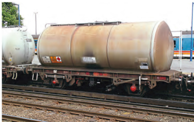
Rail traffic from the Fawley refinery used TTA wagons for various flows including diesel fuel deliveries to various motive power depots. No. ESSO 56117, photographed at Eastleigh on July 11, 2003, is the type being represented by one of the models. Again, the use of common parts means that the underframe is different to that of the model and the end ladder is at the opposite end of the wagon.
