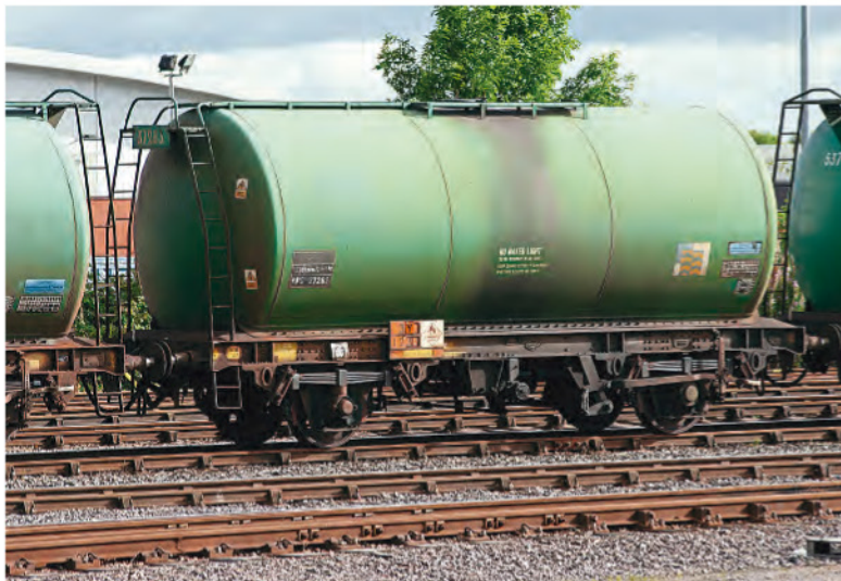
No. BPO 37263 at Inverness on August 22, 2005. This is a 1965-66 Norbitt-Pickering TTA wagon with its BP logos painted over and is the same type that the Hornby BPO-registered model loosely represents. The access ladders are mounted at the opposite end to that on this wagon type. They should be at the opposite end to the cranked brake lever.
