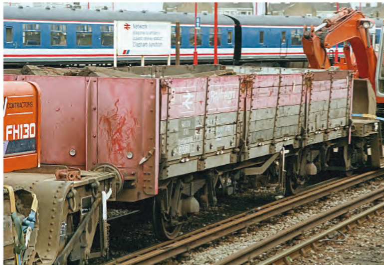
As general merchandise traffic declined in the 1980s, OAA wagons were transferred to departmental fleets and recoded as ZDA. No. 100068 carries the Fiskind name 'Squid' and was in use as a spoil wagon loaded with old sleepers on April 27, 1991. Note the red headstocks and faded condition of the wagon.
