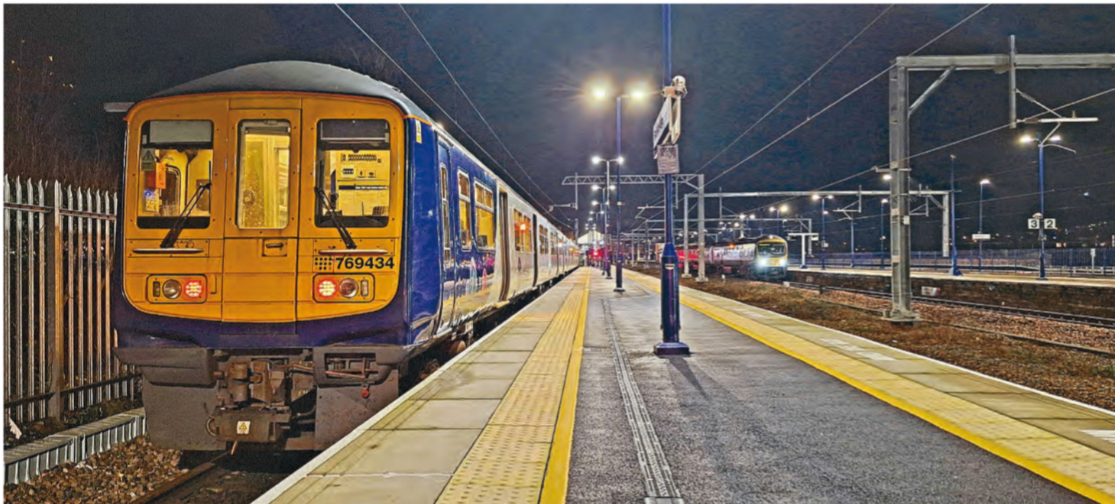
Electrification and modifying existing fleets with new technology are some of the suggestions made by the rail industry to combat the need for additional rolling stock. Northern operates eight Flex bi-mode Class 769s converted from Class 319 electric multiple units first introduced in 1988. On January 4, Northern No. 769434 stands at Stalybridge having arrived with the 2W68 19.29 from Southport, while TransPennine Express No. 185132 calls with the 1P38 19.03 Hull-Manchester Piccadilly. The station has been electrified as part of the TransPennine Route Upgrade, albeit no electric trains yet serve the station. Phil Wallis
