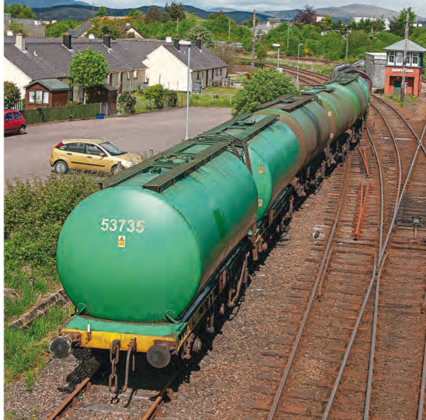
You do not need a lot of TTAs to model some traffic flows including those that ran to the small terminals at Fort William, Lairg and Oban. On May 29, 2006, the weekly delivery to Fort William consisted of five TTAs. The BPO-registered tank wagons are of different types, and this is evident from the top walkways.
