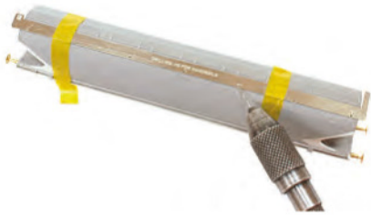
↑ Using the drilling template to accurately drill out mounting holes for the top hand rails.
