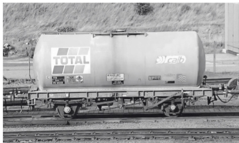
Hornby announced a Total Oil version of the TTA for 2024, to be produced in a pack of three wagons. No. PR58248 was built by Powell Duffryn in 1966 and would be a very close, if not exact match to the ESSO model. Note the pipework at the right-hand end of the wagon.
