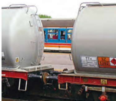
Close-up detail of the ESSO-registered wagon's end ladder detail.
