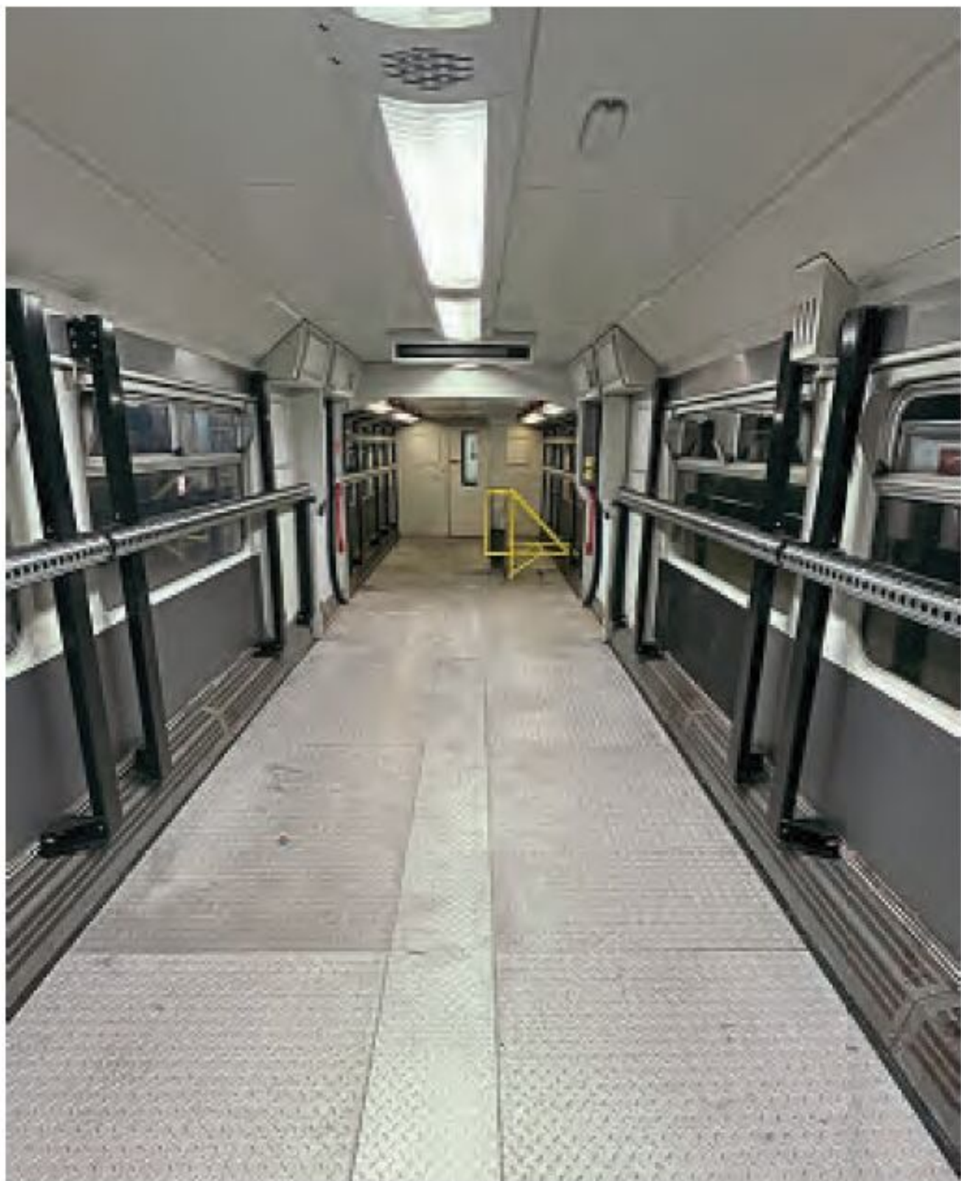
The interior of a vehicle from No. 321429 shows the reinforced floor and various equipment installed to secure the freight carried on board.
