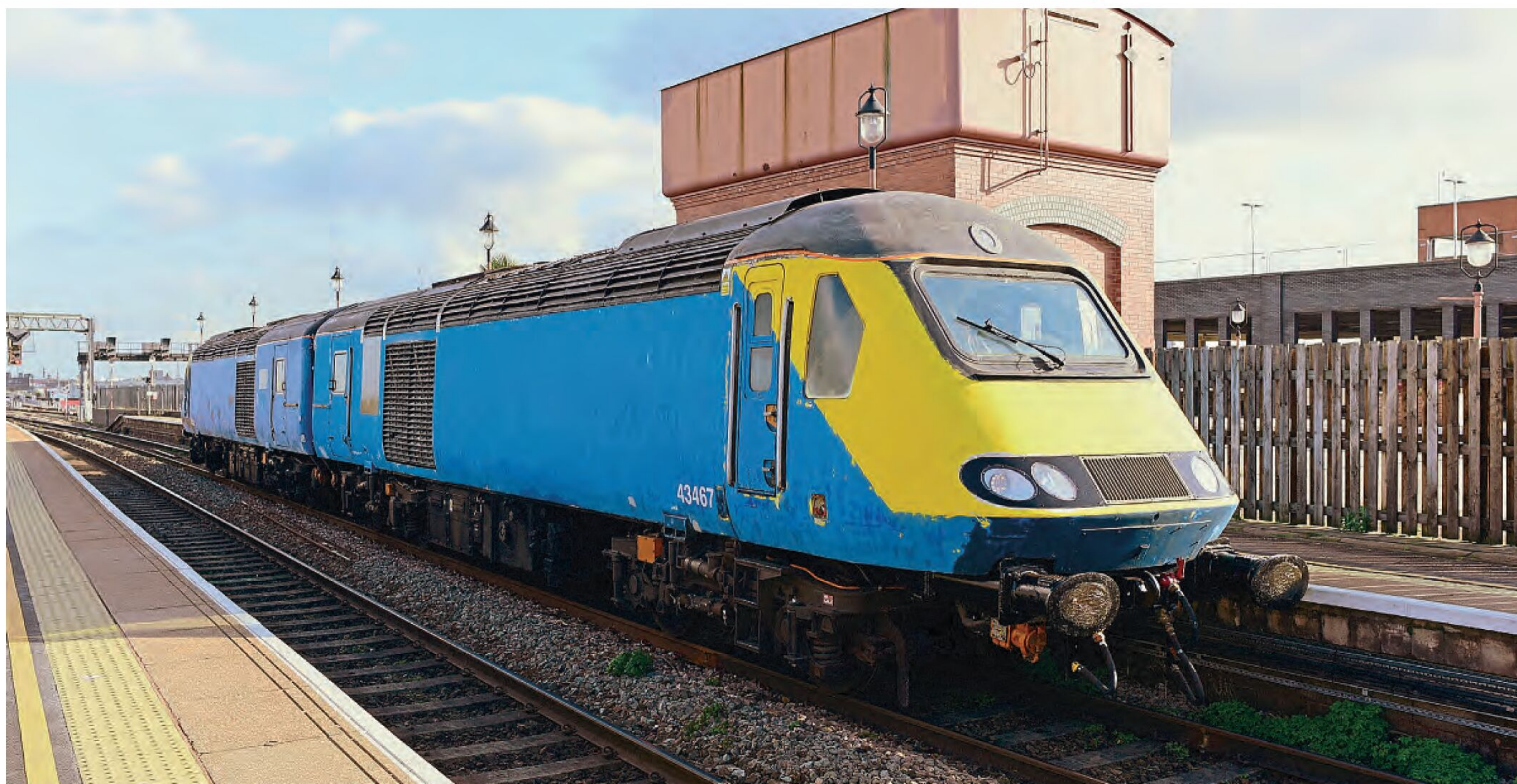
RailAdventure Nos. 43467/423 pass Birmingham Moor Street on March 5, with the 0246 14.33 Leamington Spa-Kidderminster. The '43s' were undergoing testing having received repairs at the Severn Valley Railway maintenance facility. The '43s' are destined for a return to traffic with RA, joining Nos. 43465/468/480/484. Stuart West
