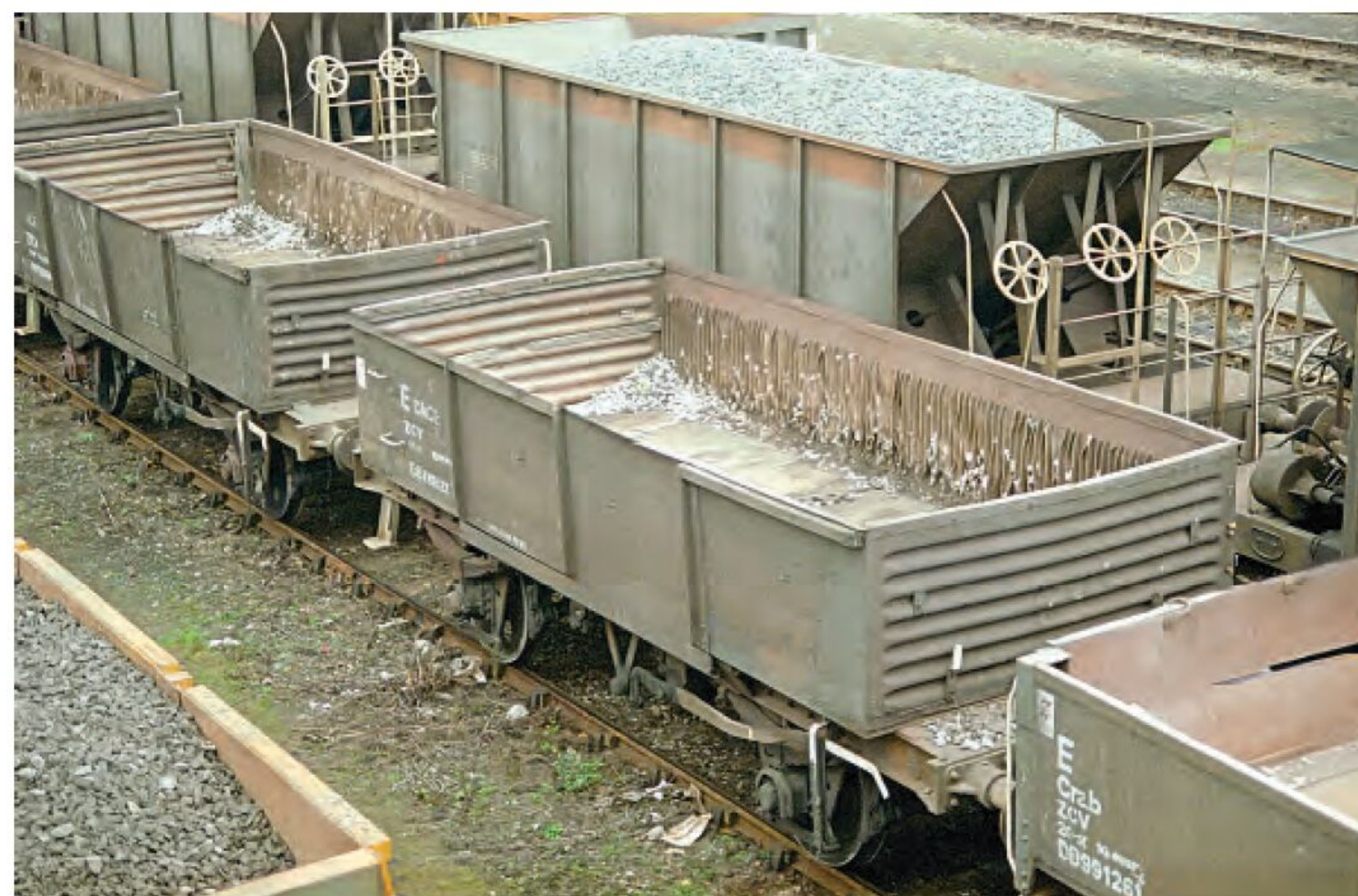
The origins of the ZCV 'Dace' wagons are traced back to the Shochood B wagons of which 300 were built at Derby in 1962 and 1963 numbered B726225-524. The original numbers were retained by the 'Dace' conversions which includes No. DB726522 photographed at Tonbridge West Yard on March 7, 1992. Note that the wooden end panelling is long gone to reveal the corrugations in the ends.
