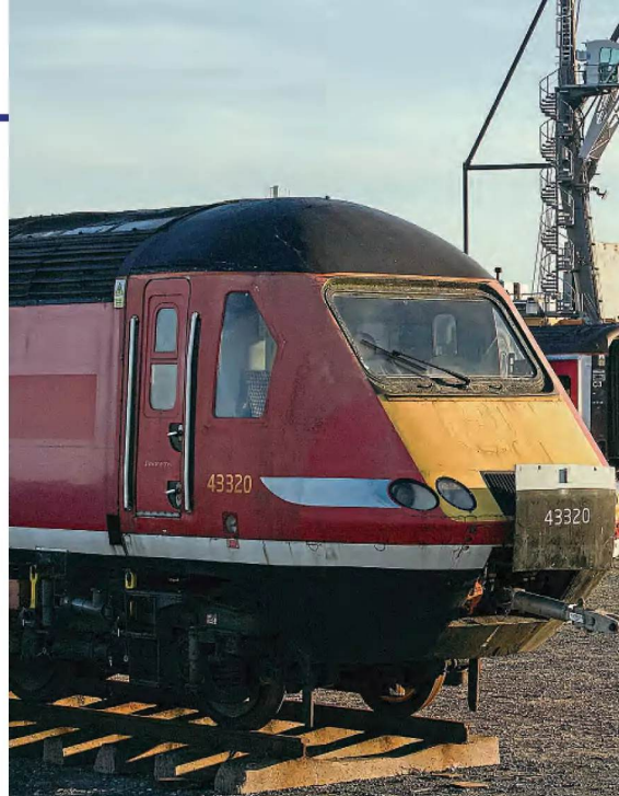
↑ Former East Midlands Railway No. 43320, one of several '43s' that transferred to EMR from London North Eastern Railway at the end of 2019, was one of the final vehicles loaded on to the MV Louise Aurebach prior to departure for Mexico. The '43' has also since hauled trains in Central America. The '43' stands on the back of a low-loader from where it will be lifted onto the vessel.
