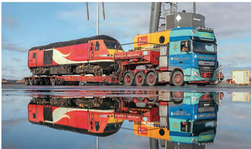
↑ Former East Midlands Railway No. 43320, one of several '43s' that transferred to EMR from London North Eastern Railway at the end of 2019, was one of the final vehicles loaded on to the MV Louise Aurebach prior to departure for Mexico. The '43' has also since hauled trains in Central America. The '43' stands on the back of a low-loader from where it will be lifted onto the vessel.
