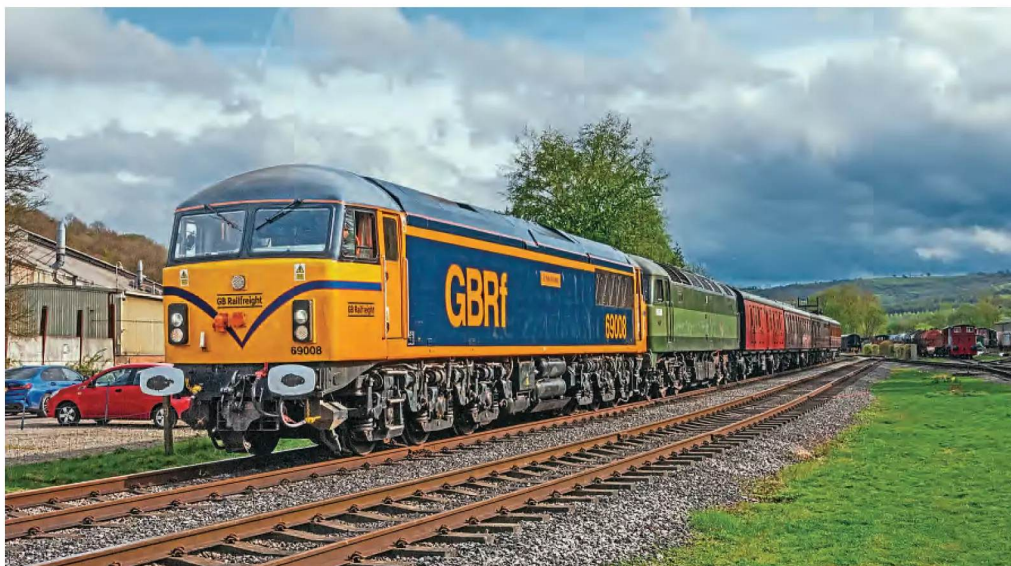
GB Railfreight No. 69008 Richard Howe (converted from No. 56038) stands at Rowsley on April 13, with No. D1501 (No. 47402) acting as a vacuum brake translator, after arrival with the 15.40 from Matlock. The '69' was attending the joint Peak Rail/Ecclesbourne Valley Railway diesel gala. Andy Flowers
