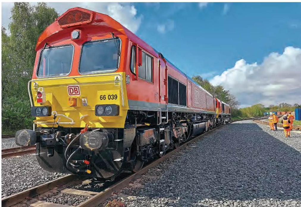
DB Cargo UK No. 66039, the first in class to be retro-fitted with European Train Control System (ETCS), leaves Progress Rail, Doncaster, on its way to the Rail Innovation and Development Centre (RIDC) at Old Dalby, on April 25. DBC No. 66183 hauled its classmate to RIDC. Network Rail
