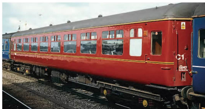
Lined maroon started to appear on West Coast Railways stock around 1998. Fresh paint was still evident on TSO No. 5487 which was recorded at Westbury on June 28, 1998. Spotting features of this stock includes the lack of a middle door and cross vestibule compared to previous builds of Mk.2 stock; larger corner doors at the coach ends and scallop roof ventilators. The lavatory windows are characterised by having small circles in the upper panes. No. 5487 has had some of the glass replaced and it is a different colour.
