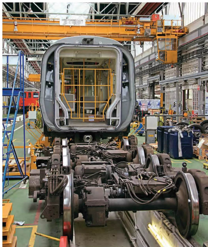
A trailer vehicle from S8 unit No. 21021/22 sits on temporary stands next to its wheelsets, which have been removed during an early maintenance programme at Neasden Dept on August 13, 2013. Note the A-Stock Rail Adhesion Train in the distance, which was retired in 2017. Christopher Westcott
