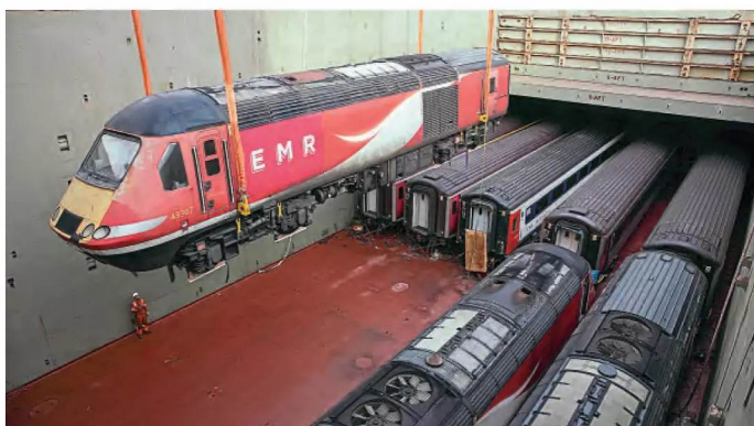
↑ The MV Louise Aurebach has several levels used to store the High Speed Train vehicles for their journey to Mexico. Former East Midlands Railway No. 43307 is lowered onto the vessel alongside two other '43s' and five Mk.3s.
