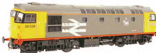
Railfreight No. 26038 is finished in Railfreight red stripe livery with features to match including the underframe air tank frame, revised cab windows and flush front.
