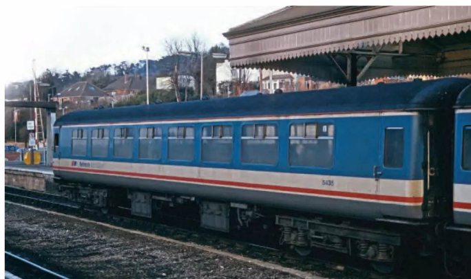
Classic Network SouthEast livery as applied to TSO No. 5435 and in use on Network Expresses between Waterloo and Exeter St Davids. Note the unpainted window dividing frames and the light shade of NSE blue. Rain gutters are red whilst the ends are painted black.
