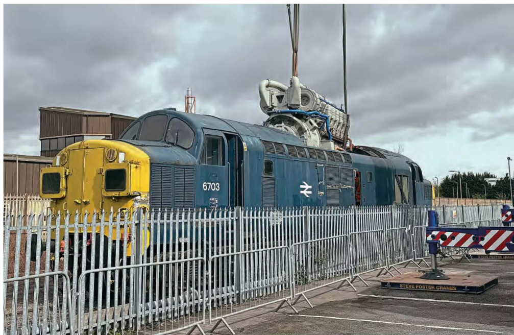
The engine is lowered into No. 37003 at UK Rail Leasing, Leicester, on April 11. The locomotive is the second-oldest surviving Class 37 and its owners plan to return it to as-built condition. C37LG
