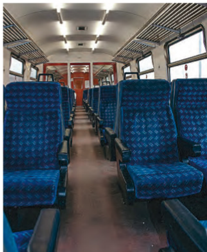
↑ The interior of the TS of No. 1531 showing Network SouthEast blue seating moquette, the fluorescent strip lighting fitted during refurbishment and orange end panels.
