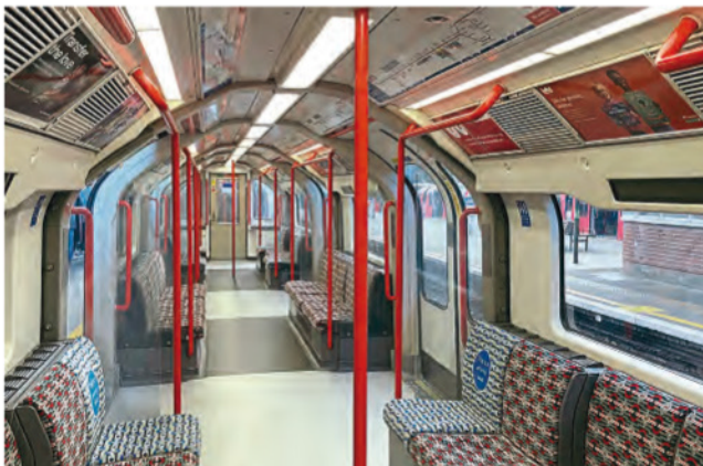
The interior of the first overhauled 92 TS unit which includes a new seat moquette. Once any changes have been made, the eight-car train will have a fresh vinyl applied prior to re-entering passenger traffic. Amir Dawoodbhai
