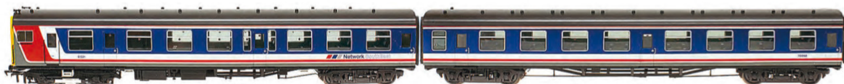
No. 1512 in its full formation with the powered DMSO to the left. The one on the right has the MG set.
