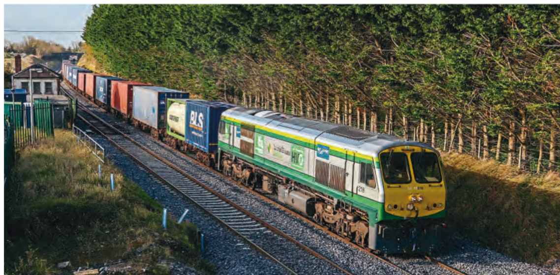
No. 218 River Garavogue hauls the 08.05 Ballina-North Wall IWT intermodal through Cherryville Junction on November 13. No. 218 is the first of the Iarnród Éireann locomotives to use hydro-treated vegetable oil (HVO). Finbarr O'Neill.
