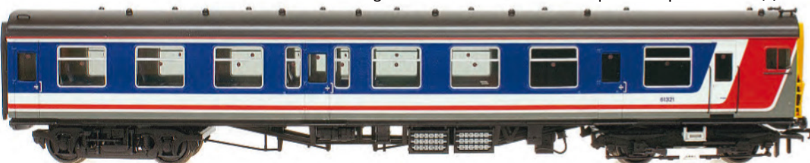
The MBSO(B) vehicle with the power bogie and internal circuit board. It carried the number No. 61321. The unit is modelled as a 1957 Phase 1 set and has shell roof ventilators and complete rain guttering.
