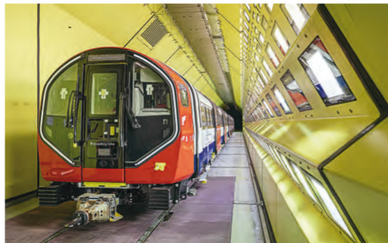
The three-car pre-production unit example, consisting of DM-IM-KM cars at the Siemens climate chamber. Siemens Mobility
