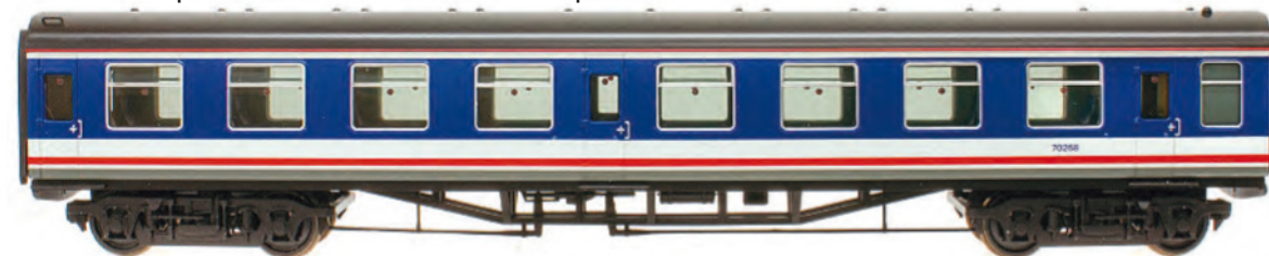
Trailer Standard or TS No. 70268. The lavatories are at the right-hand end where the coach is coupled to the powered MBSO(B).
