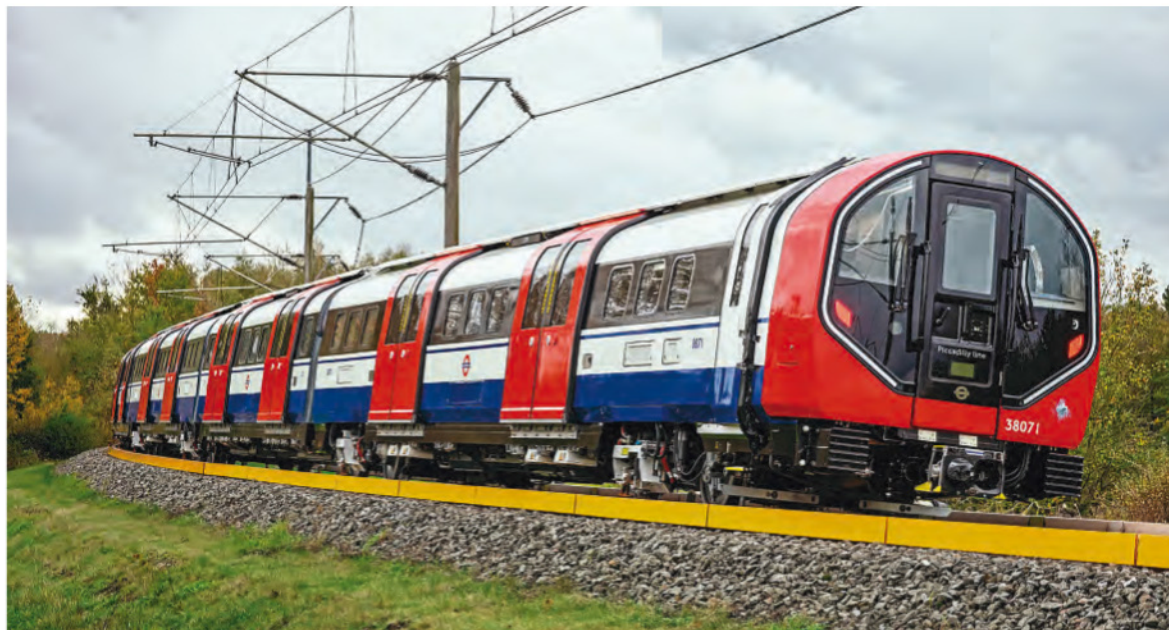
The first pre-production 24 Tube Stock unit undergoing testing at Siemen's Test and Validation Centre in Wegberg-Wildenrath, Germany. Siemens Mobility
