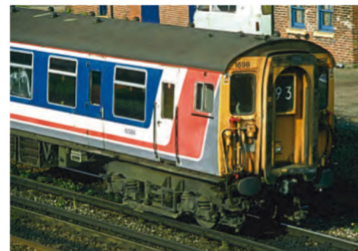
↑ 4-CEP No. 1698 is one of three units re-bogied in 1996 and was originally identified as No. 1540. They were fitted with Mk.6 motor bogies and B5 trailer bogies in 1996 in the same manner as the 4-BEPs after 1989. Intended for cover on South Central during the Class 319 overhaul programme, they worked on Brighton line services until 1998 when they were transferred to Stagecoach SWT. They retained Network SouthEast livery until 2000 and worked for SWT until 2004 when they were transferred to Connex South Eastern. They were the last 4-CEPs, albeit not instandard condition, to remain in traffic. No. 1698 was the very last one, being withdrawn in September 2005. It was photographed on June 1, 2000, at Eastleigh.
