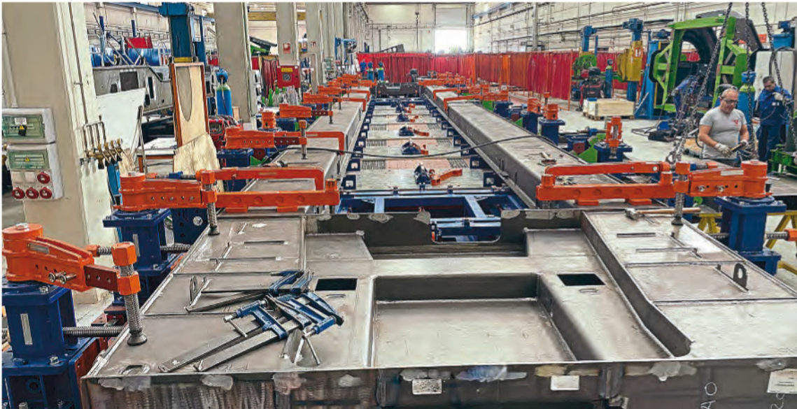
The first frame of a GB Railfreight Class 99 at Stadler's Valencia factory, in Spain, on December 18 last year. The '99s' are Co-Co bi-mode locomotives that are due to be introduced by the operator from 2025. Initially 30 have been ordered and they are expected to haul intermodal trains. They will have a 75mph maximum speed. More details on the class are expected to be revealed later this year. GB Railfreight
