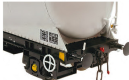
↑ Headstocks are fitted with neat models of Oleo buffers, working Instantan couplings and a single airbrake pipe.
