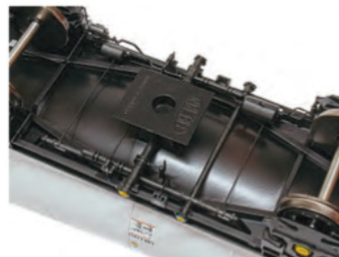
↑ The tank barrel's distinctive shape is carried through into the underframe which is detailed with the bottom discharge hatch and aeration pipework.
