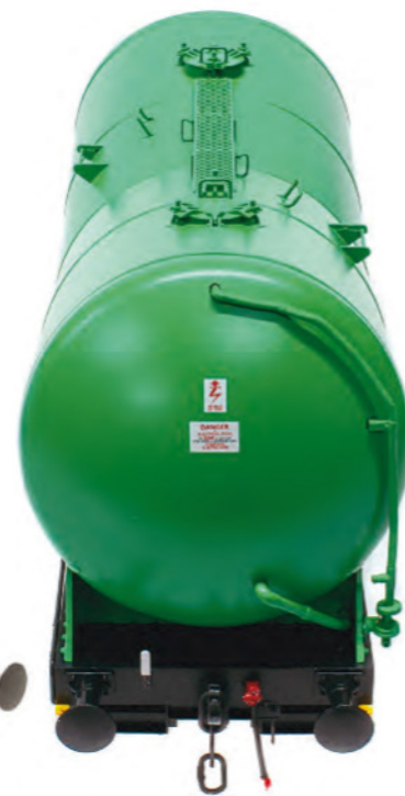
↑ An end view showing the fit of the barrel superstructure to the underframe. The warning notices on the dished ends are clearly printed and easy to read.
