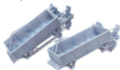
No off-the-shelf model of the ZCV 'Dace', which were used extensively on the Southern Region and in early privatisation, is currently available. A printed resin kit is available from Scale Model Innovations. Many of the spare underframe parts left over from the 'Grampus' kit can be used to finish this model.
